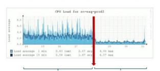
18.000 services monitoring system with Nagios core Replacement with Checkmk micro core (CMC)
